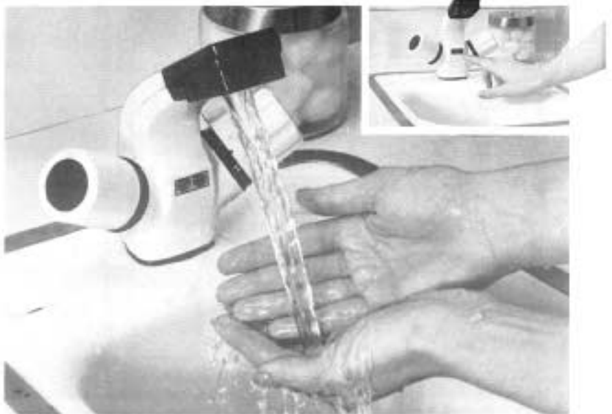
Cue-Tel bath-and-kitchen faucets turn on in presence of hand or object, turn off when it is taken away.
