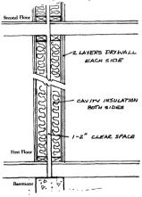
Wood framing is extremely stiff, so it transmits low-frequency sounds and impact noises well. Resilient channels or a double wall with a one- to two-inch clear space between are the best solutions for woodframed party walls.
