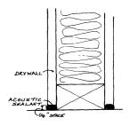
Acoustical sealants are used to seal up sound leaks at partition tops and bottoms electrical outlets, and other penetrations. Any flexible, non-hardening sealant will do
