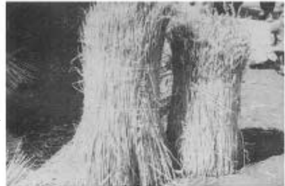
Combed wheat, pictured here, is one of three popular thatching materials. The others are long straw and water reed.
