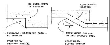
up, its bottom should rise along the angle of repose.
