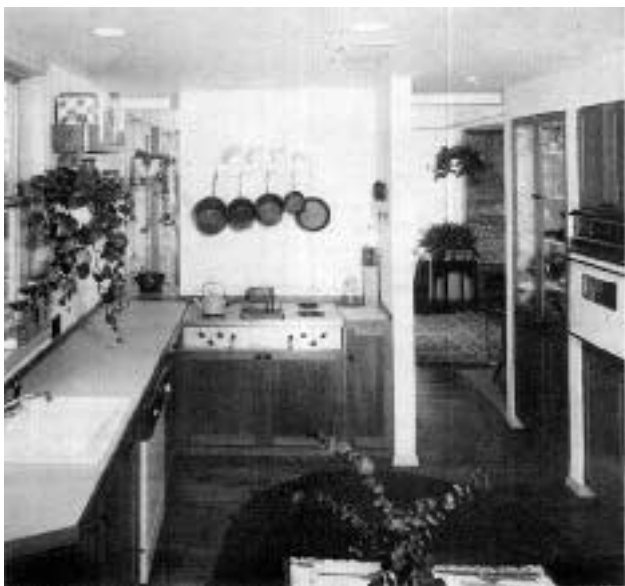
Recessed downlights provide ideal lighting in a kitchen with no wall cabinets over counters. With standard wall cabinets, some form of under-counter lighting is needed.
