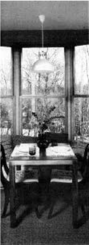
The only place to use hanging fixtures is over a table or in a high space such as a stair hall where the ceiling needs to be visually lowered.
