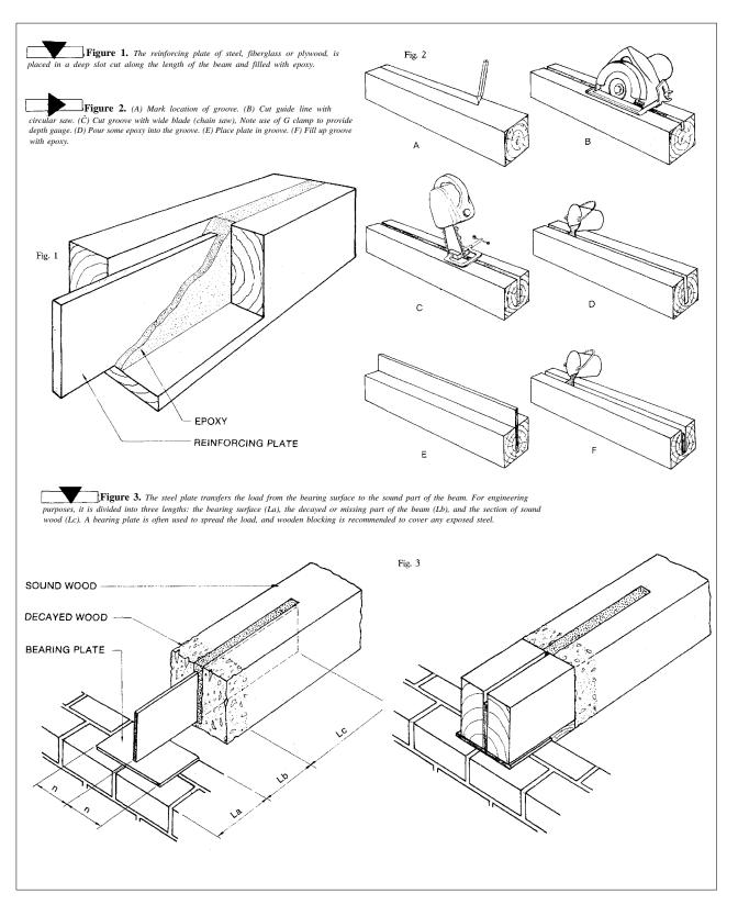
The WER system is designed to reinforce deteriorated timbers. It is not a wood preservative. Therefore, after the wood is reinforced, you must brush it generously with a preservative to prevent further decay
