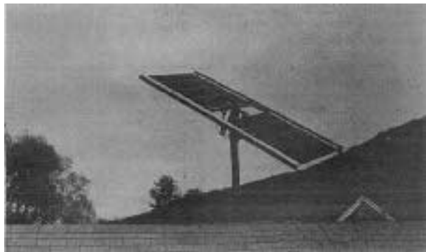
This pole-mounted Zomeworks tracker takes full advantage of the sun by moving east to west with the day's light.
