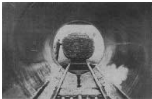
A treating cylinder at a lumber-treating plant about to receive a load.
