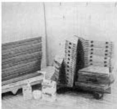
Cut on the author's radial-arm saw, all the pieces lay ready for gluing with West System epoxy.
