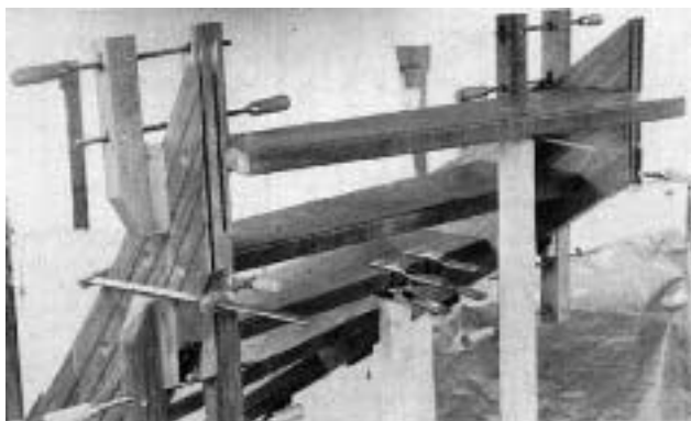
While a bar clamp applies pressure to close up the joints (above), two hand-screws with beveled jaw-pads clamp the cheek of the mortises. The finished joint (left) contrasts the butternut stringer with walnut splines.
