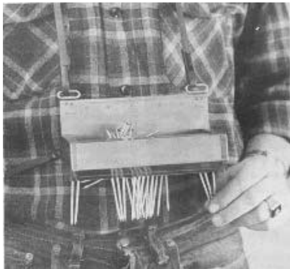
Tools of the trade: A nail stripper (left) can greatly speed up shingling. (Made by McGuire-Nicholas Mfg. Co., 6223 Santa Monica Blvd., Los Angeles, CA 90038.) The shingle hatchet (above) has a blade for trimming, and a shingle gauge for checking courses.
