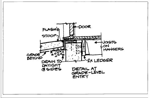
such as W.R. Grace's Bituthene. The trap here is that the bottom of the flashing must drain decisively away from the building. Otherwise, water will simply collect underground and rise up underneath the flashing, saturating the sill, band joist, and joist ends, with disastrous results. However, this approach is the only one available in renovations, where the foundation is already in place.
