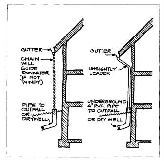
my last house design). If the door is under an eave, whether overhanging or not, it is essential to provide a gutter or diverter to keep the entry from doubling as a brief showerbath during rains. Make diverters substantial, at least 1½ inches high, and make them sturdy. Copper wrapped around a triangle of treated wood attached through an uphill flashing flange works very well.
