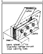
The resulting composite can be very helpful where you can't easily fit a full-sized wood beam.
