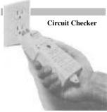
Hand-held circuit analyzer detects voltage drops that exceed the limits set by the National Electric Code.
