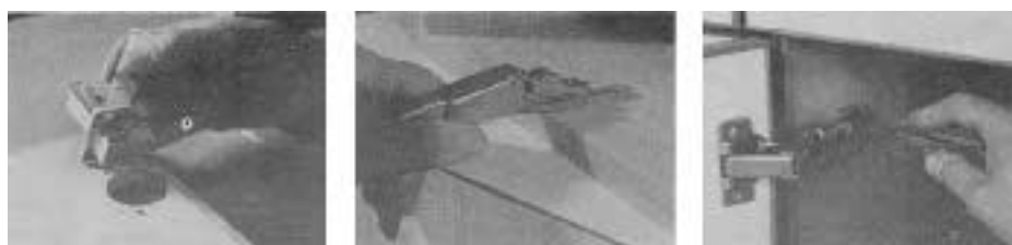
Figure 7. Mounting cup hinges is simple: First, bore a 35mm-diameter hole on the inside of the cabinet door. Press the hinge cup into this mortise (left), which holds it tightly in place until the hinge is screwed in. Next screw a base plate to the inside of the case (center). Finally, slide the hinge over the base plate (right); a single mew locks it in place.
