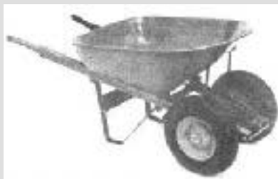
Make sense to you? It does to us, but unfortunately the company that used to make this two-wheeler has gone out of business. A two-wheel wheelbarrow may look odd at first, but users say it provides more stability for heavy loads.
