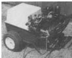
Small commercial applicators can purchase spray equipment for bleach or preservatives from lawn-care or golf-course suppliers. This unit is the Suburban Sprayer from Weatherguard Systems, Inc., in Marshall, Texas.
