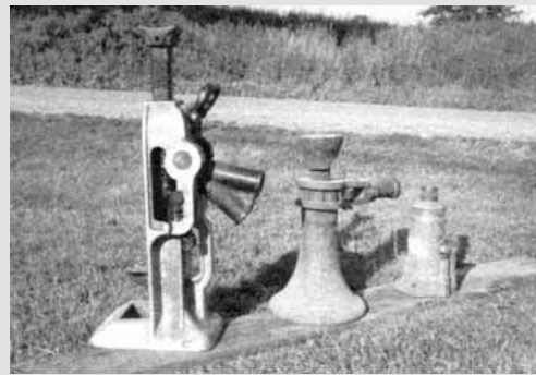
Figure A. Shown left to right are a railroad jack, a screw jack, and a hydraulic jack. A fourth kind — the adjustable floor post — is shown in Figure 4 (last page).
