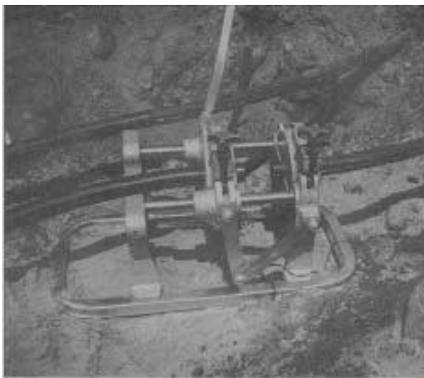
The butt-fusion fixture shown here is the proper tool for joining polyethylene pipe for use in a ground loop.
