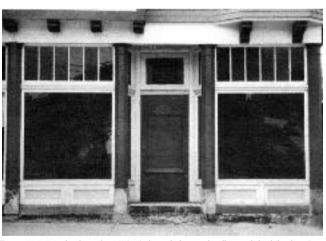
Figure 7. A "simulated storefront," (top), has a dark painted wall sitting behind the glass. It maintains the spacing of windows and entrances along the street (bottom), but makes the tenants feel more secure.
