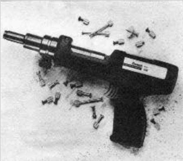
The commonly used, low-velocity fastening tools come in single shot (above) and semi-automatic versions.
