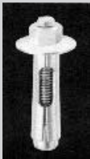
The holes for the sleeve anchors can be drilled with brackets in place (above left). Tightening the nut draws the cone up, expanding the sleeves walls (above right). As the load pulls on the stud of the sleeve anchor (right), it sets the anchor more firmly.
