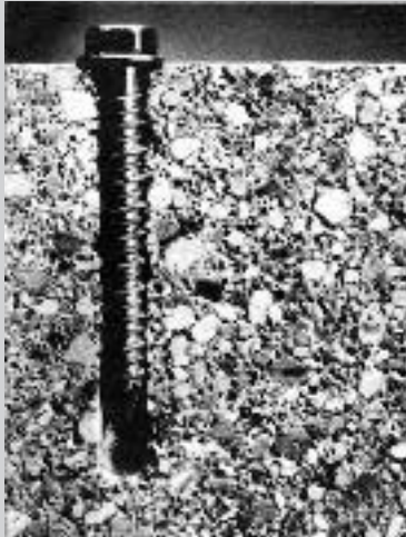
Screw anchors (right) provide their own holding power by tapping into the masonry material. The anchors (below) are threaded into a pilot hole using a screw driver or power tool.
