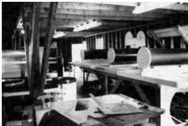
A five-person crew produced five solar hot-water heaters a day, each costing $150, at this Crystal City, Texas, factory. Recycled fluorescent bulbs and printing plates served in the collector.
