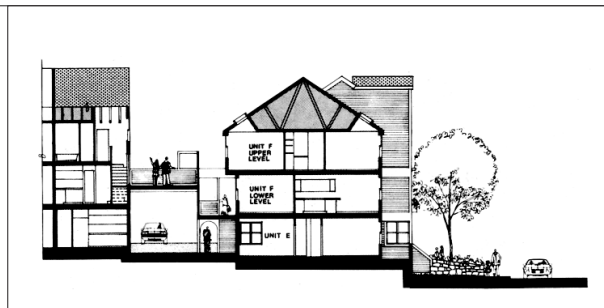
Figure 1. The arrangement shown here, a duplex over a flat, allows for a great deal of living space to be concentrated in a small area, while preserving privacy and quality of living space.
