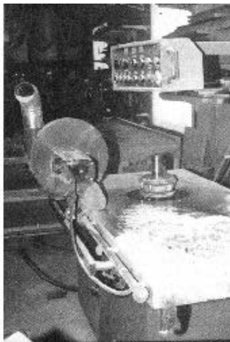
▲ Figure B. The dowel-boring machine drills holes in precise locations on the end of the panel.
