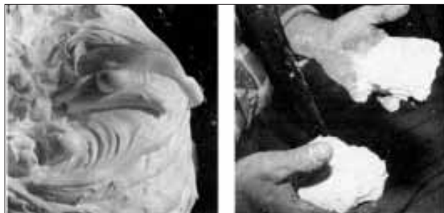
Figure 1. Puffed up like shaving cream (left), Air-Krete doesn't look anything like its cement components. After it dries a little (right), it looks more like angel food cake.
