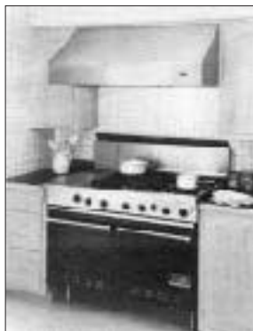
The Viking range shown above is one of a new generation of "professional" stoves designed for the residential market. It is not subject to the 6- to 10-inch horizontal clearance from cabinets that is required—but too frequently ignored—for uninsulated commercial stoves.
