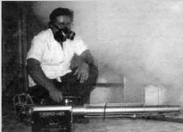
This gasoline-powered "thermo fogger" helps neutralize smoke odors. Smaller electrical models are also available.
