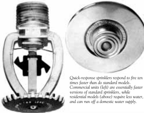
Quick-response sprinklers respond to fire ten times faster than do standard models. Commercial units (left) are essentially faster versions of standard sprinklers, while residential models (above) require less water, and can run off a domestic water supply.
