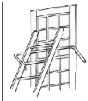
Figure 2. Handy accessories like this ladder stand-off can make ladder work safer and easier.
