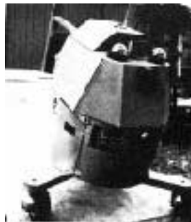
"Kluge" was developed by Cybermation Inc., in Roanoke, Va. It is a radio-controlled, three-wheeled machine that can navigate tight passageways.
