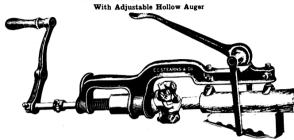
This machine is now made in two sizes. One size cuts from  $\frac{1}{4}$  to  $\frac{1}{4}$  inches, the other from  $\frac{1}{4}$  to  $\frac{1}{4}$  inches. They are guaranteed to give satisfaction. The auger head is extra heavy. The knife starts on the blunt end of the spoke, and centers perfectly. The auger is kept cutting by the force of the spring. It is adapted to any size spoke or dish wheel.
