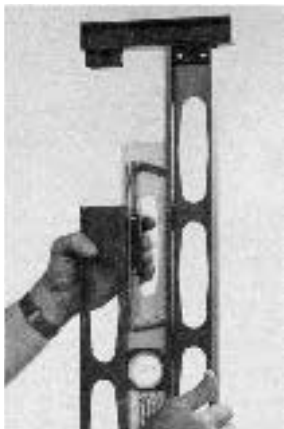
Plumb-It, invented by Paul Semler, consists of a level flanked by two aluminum I-beams that ride up and down on the level's flanges. The popular 4-foot version can be expanded to 10 feet 8 inches with no play.
