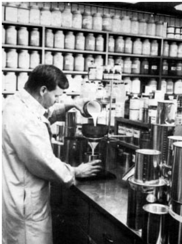
Traditional oil paints mix small amounts of heavy resin with large volumes of solvent. Now paint technologists need to make low-viscosity resins work with little solvent.
