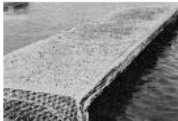
This wire mesh form shows the very early deposits of minerals that have been drawn out of seawater by a low-level electrical current in a process called accretion. Soon this form will accumulate enough mineral deposits to make a wall panel that will have a 4,200 psi rating.
