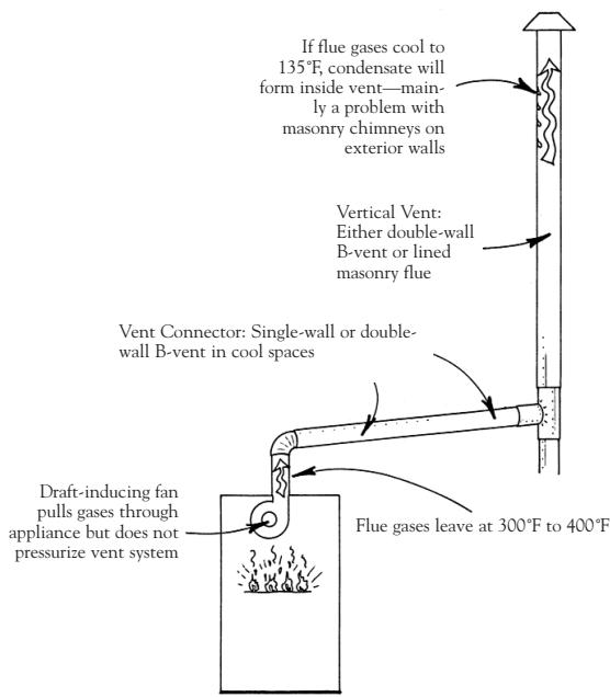
Flue gases from mid-efficiency "induced-draft" gas appliances can condense in the venting system and lead to corrosion. To prevent such problems, both the vent connector and vertical vent should be sized properly (not too large) and preferably use double-wall B-vent. Despite the exhaust blower, these appliances still rely on natural draft for venting.
