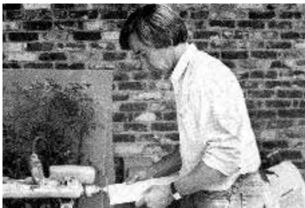
Figure 1. Unlike ceramic tile, exposed edges in marble and granite tiles have to be fabricated with grinding and polishing equipment. Here, Duncan polishes a standard flat edge on a marble tile using diamond pads chucked in a drill motor.
