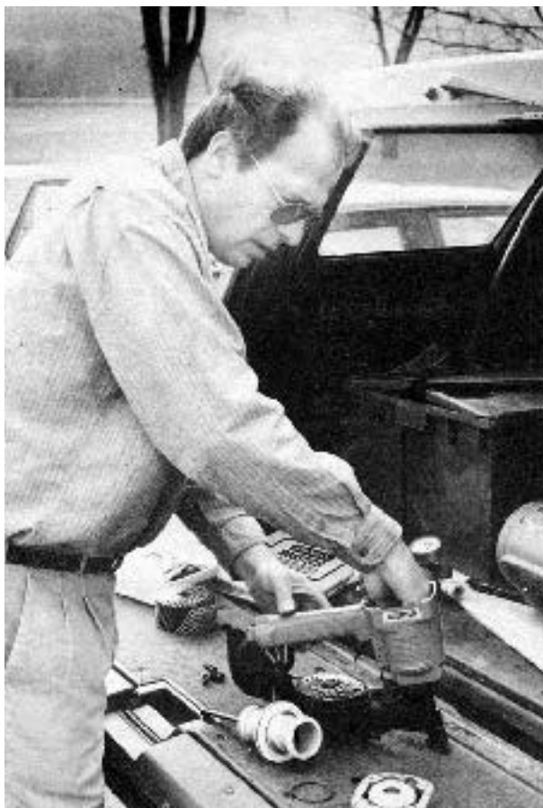
Pneumatic nailers rely on the physics of air to operate. Mechanically they are simple tools; cleaning and light repairs can often be handled at the site on the tailgate of a truck.
