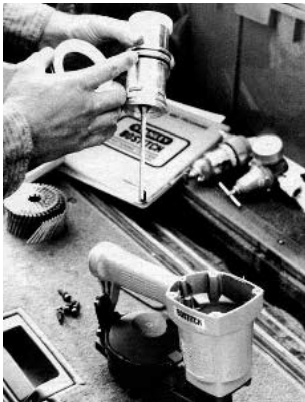
Figure 3. O-rings, such as the main-cylinder seals pointed out in the photo, fit tightly in tracks to seal the chambers inside an air gun. Handle O-rings with care since any debris in the track or on the ring will ruin the seal.
