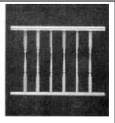
**Pre-fab stair rail.** Assembling open stair railings takes time, even when you aren't making the parts. So, Morgan Products came up with a pre-assembled balustrade called Rail Easy, shown above. Sections of rail join to newel posts (starting newels, landing newels, half newels, and intermediate newels) with a shoulder screw that creates a tight, secure joint tested for loads of over 250 pounds.
