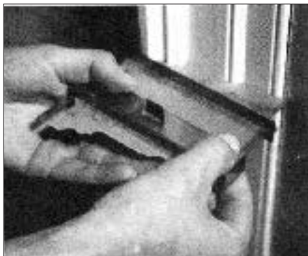
Figure 4. You can copy a molding profile with a profile gauge, a row of slender pins held loosely in a frame. The pins lock in place allowing you to transfer the shape.
