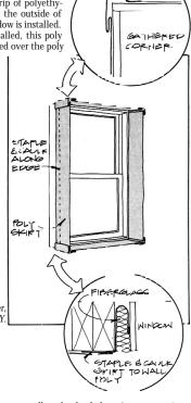
**Rubber gaskets.** The bond between caulk and polyethylene (even expensive acoustical caulk) has questionable reliability. So this detail was devised to avoid caulk altogether. It uses specialized EPDM rubber gaskets in place of a skirt and caulk. The product, called *Gap-Gaskets* can be purchased for about 60° per linear foot from Resource Conservation Technology (2633 N. Calvert St., Baltimore, MD 21218; 301/366-1146).
