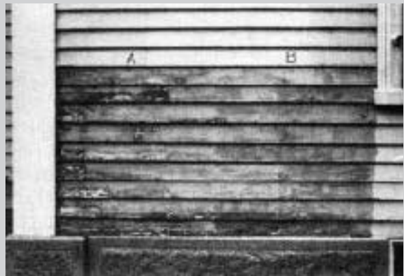
Figure A. Two 3x3-foot test panels show the results of different removal methods. The panel on the left, marked "A," was cleaned up with a heat gun. The 3x3-foot section to the right, marked "B," had paint removed using a heat plate with heat gun cleanup.
