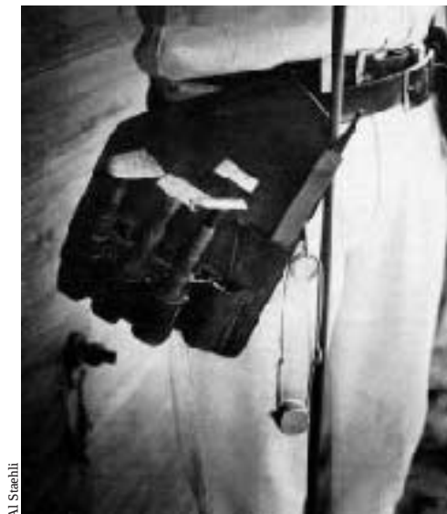
Figure 4. Bell manufactures its own contoured scrapers and tool belts. A file is carried to keep the tools sharp.
