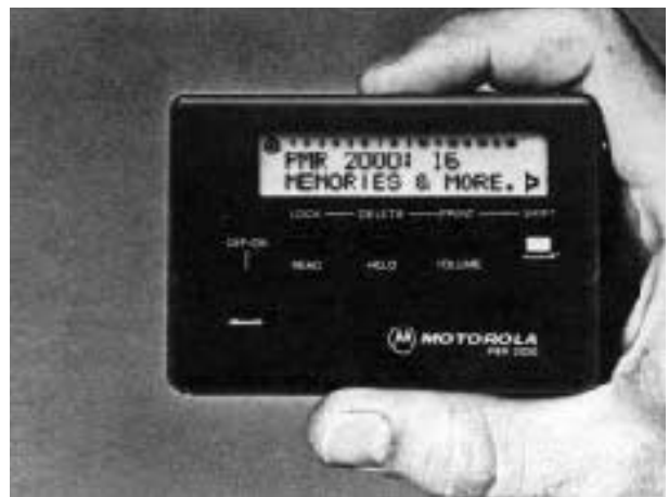
Figure 3. This top-of-line pager—or personal message receiver—can pass any combination of tone, voice, or alphanumeric messages, including continuous "scrolled" messages that roll up the screen. It can store up to eight messages, and with an optional printer, it can even print out a message up to 1,950 characters long. If you don't want an annoying beep, it can alert you to a call by vibrating.
