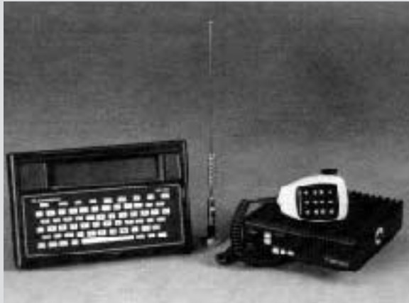
Motorola's mobile data unit lets field personnel access and input information from a central computer via the two-way radio.
