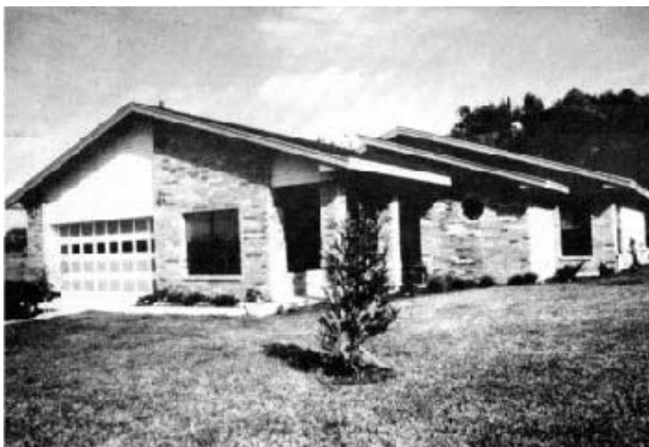
The exterior of this steel-framed home looks like any other. It uses OSB or plywood sheathing over steel studs and can have any kind of siding, including brick veneer.
