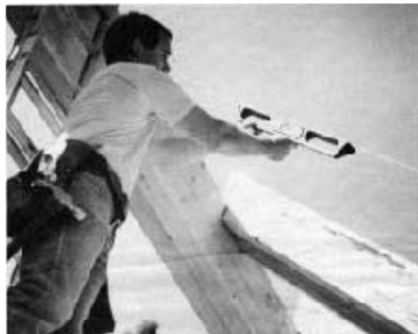
The Smart Level precisely measures angles between 0% and 90% — in addition to level and plumb. The LCD readout remains upright even when the level is flipped over.
