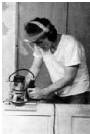
Figure 1. The Hinge Mate-1100 sets up quickly, but must be moved for each hinge.
