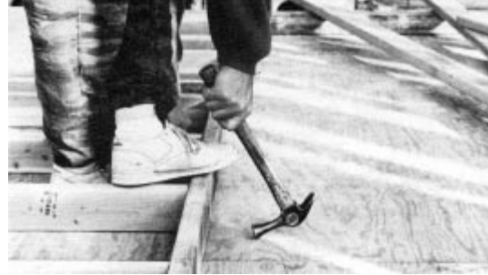
The Dogyu hammer is guaranteed to draw comments for the first time it's seen on a job site. This Japanese import has excellent balance, a standard millface, and weighs in at slightly over 20 ounces. It's a little light and a little short in the handle for some framers, but it has a lot of fans when it's time for pick-up work.
