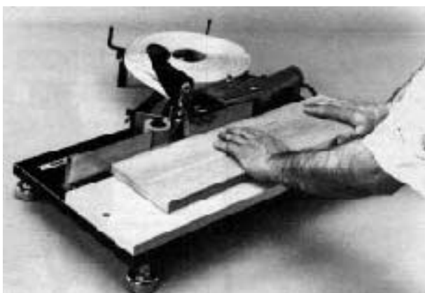
Figure 4. The Freud EB-100 edge bander applies hot-melt, adhesive-backed veneer strips to the edges of plywood panels.
