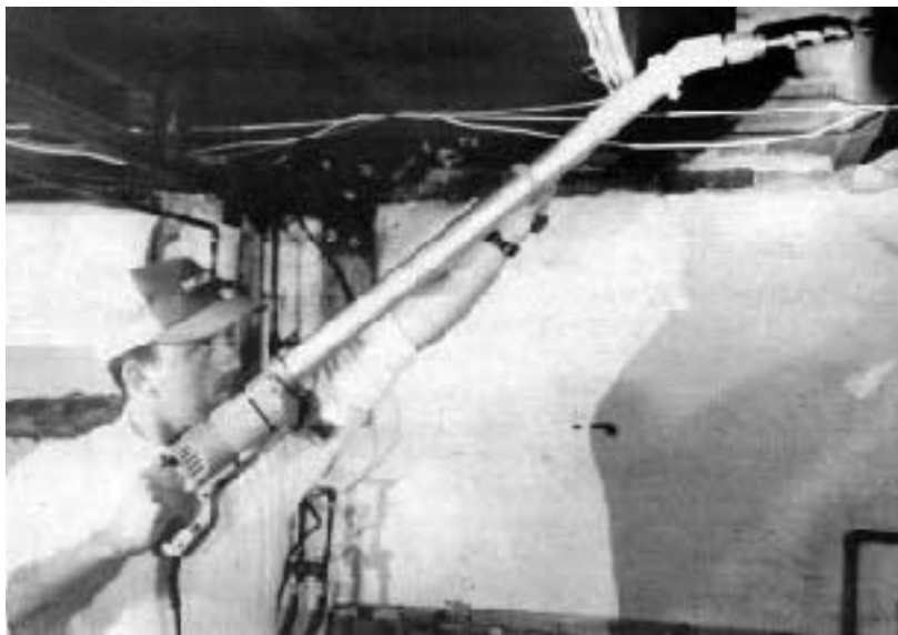
Figure 1. Milwaukee's 33° angle drill extension simplifies repetitive drilling and hard to reach electrical and plumbing work.
