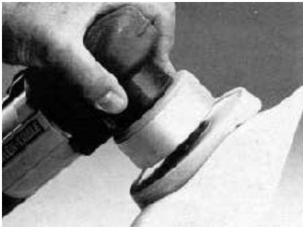
Figure 7. The Porter-Cable 7334 is the first electric-powered random orbit sander. This sander, shown here with an optional pliant pad for contoured surfaces, accepts standard 5-inch-diameter sanding discs.
