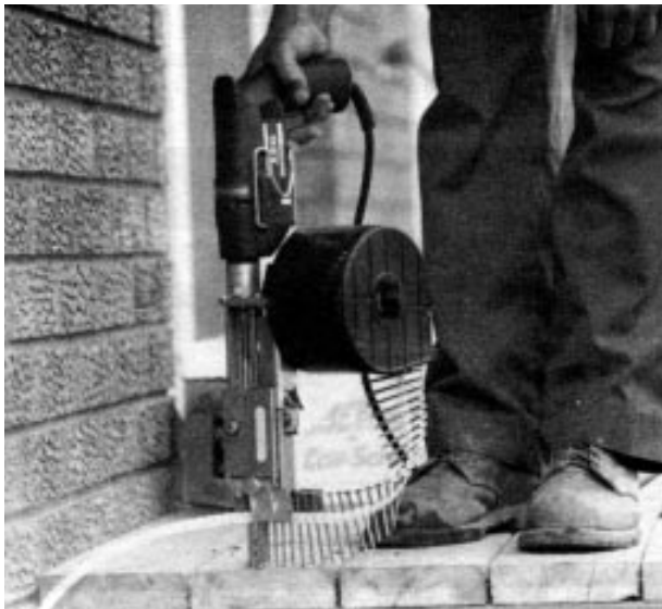
Figure 5. The Quik Drive self-feeding screwgun, holding a coil of 167 screws, can pay for itself by speeding up many fastening jobs.
