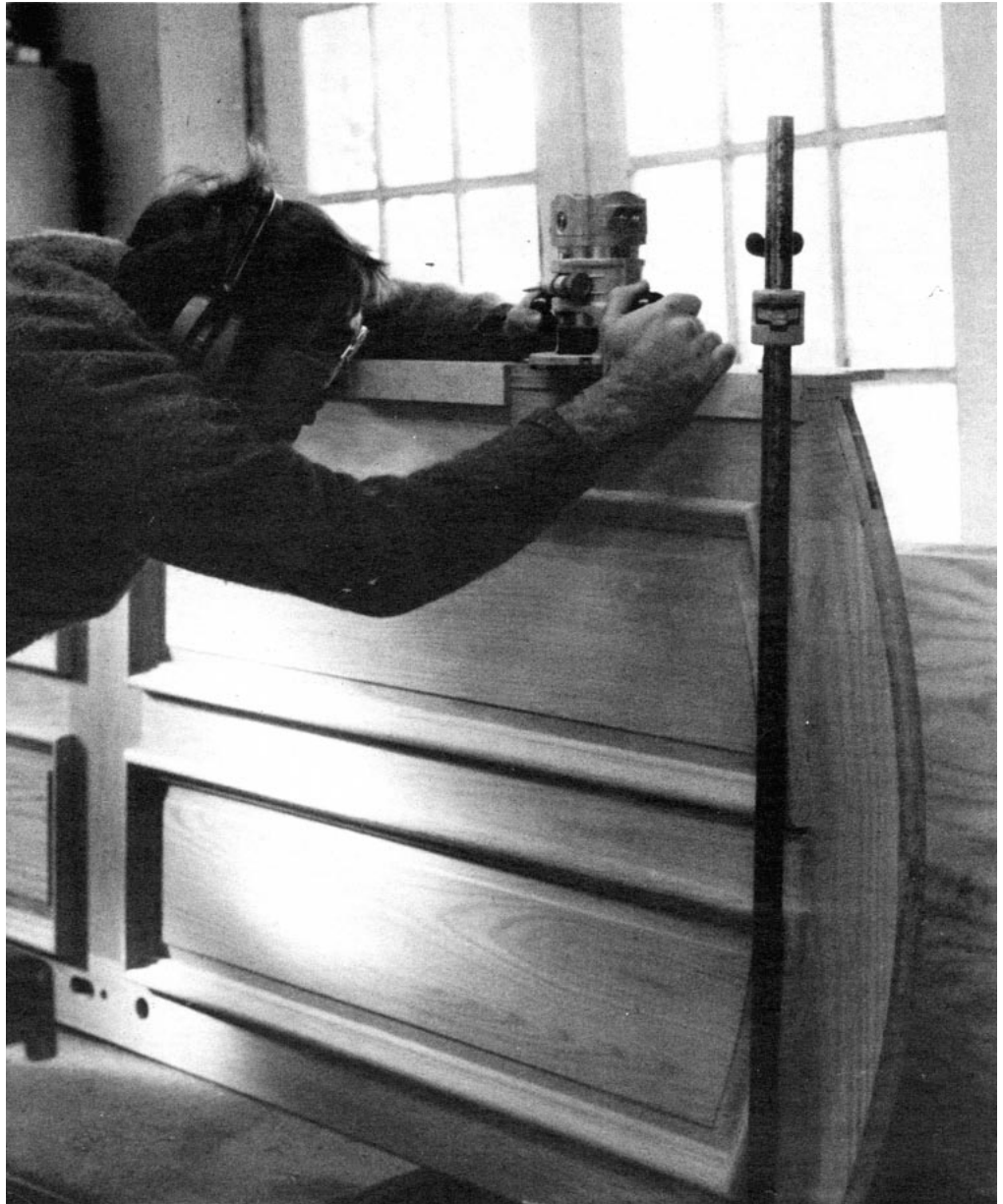
Doormaker Grant Taylor mortises a jamb with a jig made from scrap plywood.
