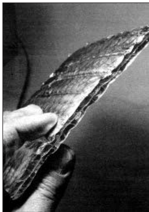
Bubble-pack insulation has a polyethylene core and foil facers. Despite some differences in thickness and makeup, all brands have similar thermal performance.
