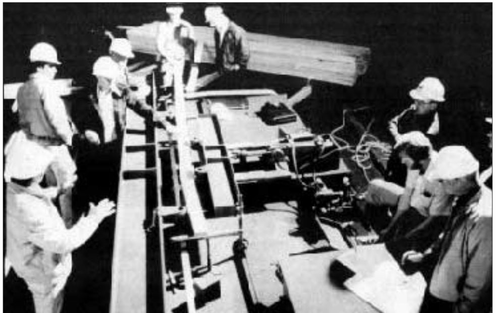
A roomful of In-Grade engineers look on as a 2x4 is tested to destruction.
