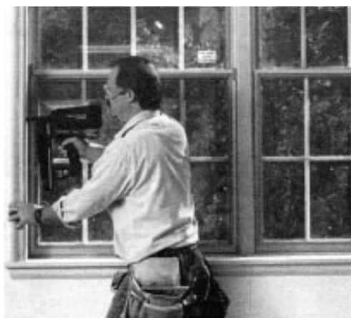
The Impulse 250 finish nailer is cordless, and will drive 3/4- to 2 1/2-inch nails, making it one of the most versatile power nailers available.
